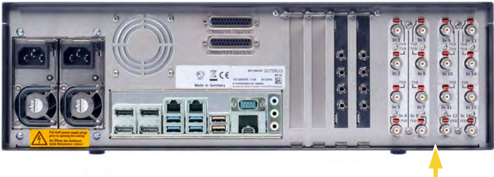
Figure: AnalogKit-H16 BNC input sockets and Audio Line In
