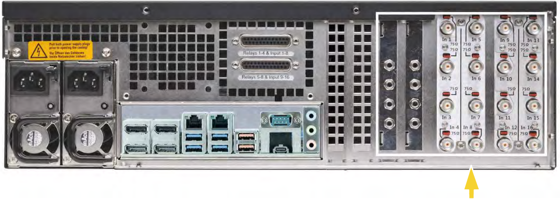
Figure 5: AnalogKit-H16 BNC input sockets and Audio Line In
