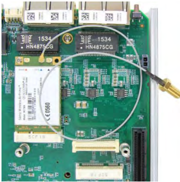
Clip on IPEX-to-SMA cable
