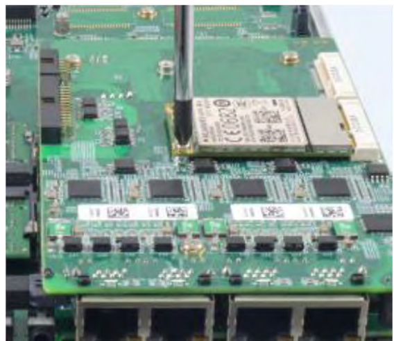
Secured with M2.5 P-head screw
