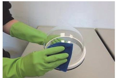
Then rinse the dome surface with cold water and dry it with a dry microfiber cloth.
