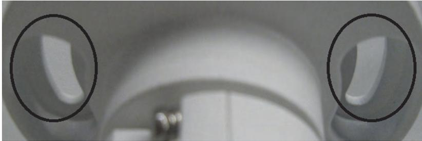
Drill two holes into the wall and press the plastic anchors (accessory bag) into them. You can choose, whether you pull the breakout cable through a third hole in the wall or use the outlet of the camera socket (then you have to ensure that the cable is placed into an IP 66 box). Take two screws (accessory bag) and fix the camera onto the wall.
