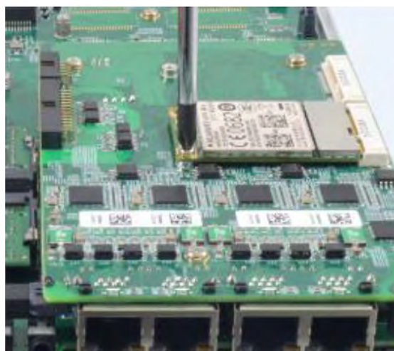
Secured with M2.5 P-head screw
