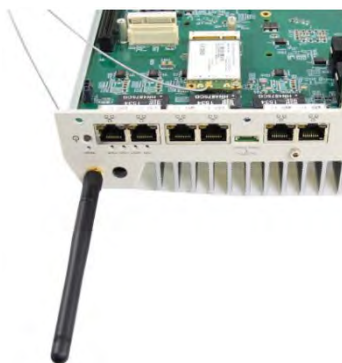
Attach antenna to panel
