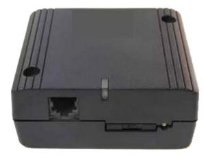
GSM Modem has to support AT commands for sending short text messages. As mentioned above, GSM Modem needs a SIM card and this SIM card has to be inserted into GSM Modem.
