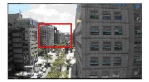
Users can configure up to 10 sets of Motion Detection Windows in each set of Motion Detection Setting. Click on the <add> button under the Live Video Pane to add a Motion Detection Window. To cancel a Motion Detection Window, move the mouse cursor to the selected window, and click on the <delete> button.
