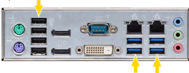
Figure : Prises USB (4x USB 2.0, 4x USB 3.0)
