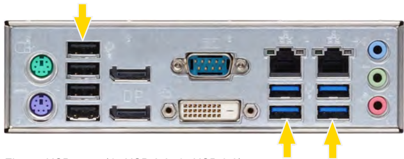
Figure: USB ports (4x USB 2.0, 4x USB 3.0)
