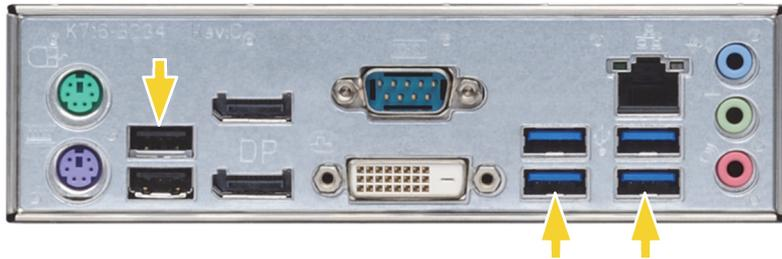
Figure 8: USB ports (2x USB 2.0, 4x USB 3.0)
