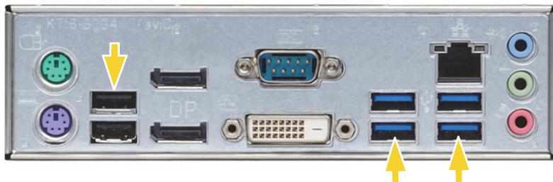
Figure 6: USB connections
