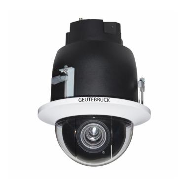
The Speed Dome camera with Full HD is suitable for indoor use. With the 360 degree panning and freely controllable lens with a tilt range from -20 to 100 degrees, gives you the optimal overview. In addition, 256 fixed positions can be set, which allows a targeted control of certain scenes. With the 30x optical zoom, distant areas do not go unnoticed and can be controlled in the usual high quality.
