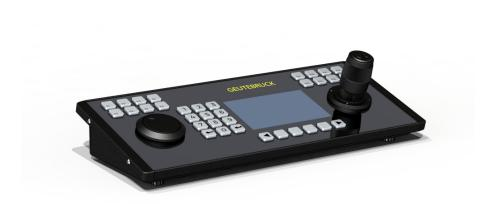
The control unit provides the user with tailor-made control of the proven Geutebrück technology. The individually configurable multi-touch color display as well as freely programmable function keys enable clear operator guidance so that the user has all situations under control at all times. The MBeg+ can be discreetly installed in table tops.
