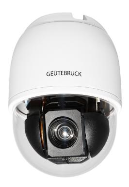
The Speed-Dome Camera with Full HD resolution is suitable for outdoor use. With the 360 degree panning and freely controllable lens with a tilt range from -20 to 190 degrees, gives you the optimal overview. In addition, 256 fixed positions can be set, which allows a targeted control of certain scenes. With the 40x optical zoom, distant areas will not be unnoticed and can be controlled in the usual high quality.
