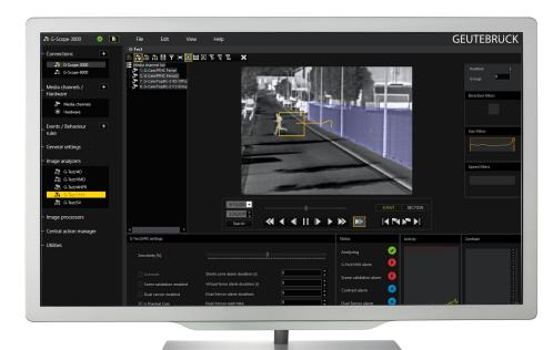
This option enables comprehensive VMX video analysis. It is characterized by high precision and reliability. With a virtual 3D model of the area to be secured, objects can be detected with exact perspective and the false alarm rate reduced. This makes this video analysis particularly suitable for perimeter monitoring.
