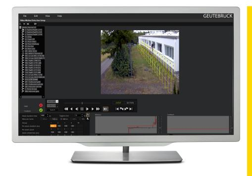
This option provides 3D video motion detection. These are characterized in particular by high reliability and precision, making them particularly suitable for monitoring critical outdoor areas. By detecting perspective differences, objects can be reliably detected in real time according to size, direction and speed.
