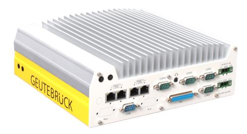
The hardware platform is designed for mobile use and guarantees optimal interaction with Geutebrück software. The certified construction can be used in vehicles of all kinds and can also be connected via wireless transmission (WLAN, mobile radio). Due to the special design, the hardware is passively cooled and requires no active cooling. The device has four network ports (PoE+). Please note: The parameterization of the system determines the required hardware resources.
