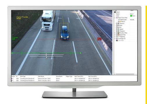
Camera-based video content analysis is an elementary tool for video surveillance. With the VCAcount option you can keep track of passenger flows and road load factors. Counting of people or vehicles can be realized in an instant using the People Counting function and easy configuration.
