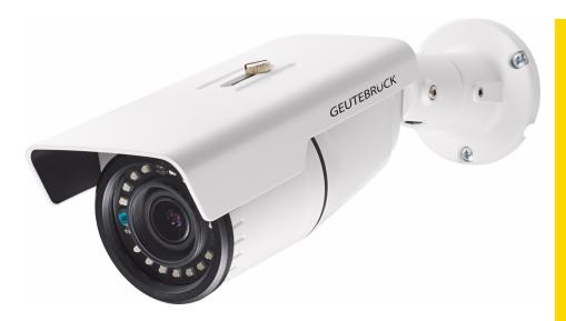
The Bullet Camera in Full HD resolution is optimally protected of weather, sunlight and vandalism by a weatherproof housing with built-in sunshield. The lens is perfect for monitoring the immediate surroundings and provides sharp images even at night thanks to the integrated infrared LEDs.
