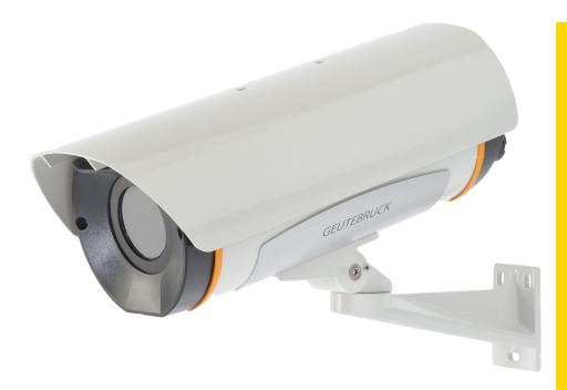
The Thermal Camera enables observation in very low light or rough terrain. With a frame rate of 30 Hz for a smooth image flow and a viewing angle of 24 degrees, it is possible to detect people up to 160 metres away. The weatherproof housing offers perfect protection against weather and sunlight.
